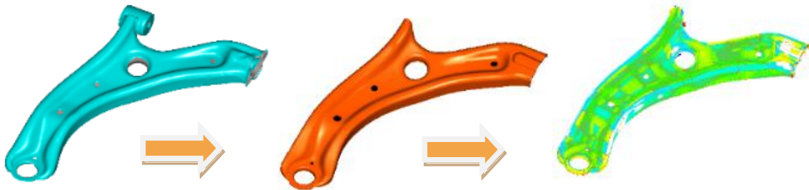
3D Scan as a polygon model Automotive Suspension Arm
